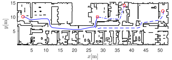
Fig. 15. Three planned paths at the department map obtained by the HE* algorithm. The start of each trajectory is noted by o-mark and a common goal by \square -mark.
